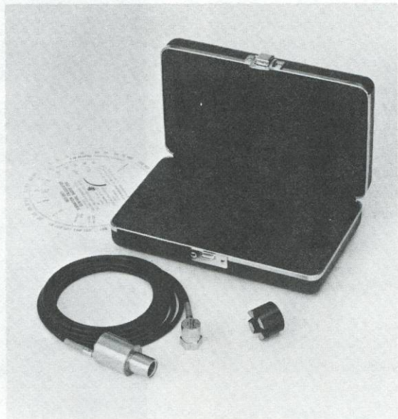
Figure 6-19. Vibration integrator system.
